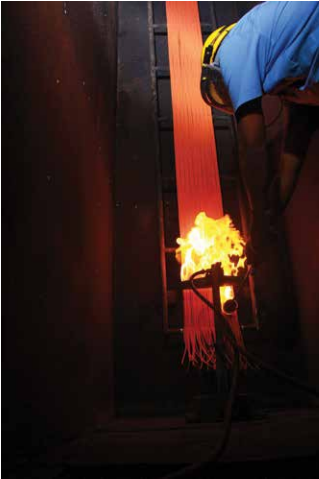
Testing of vertical flame spread of low smoke halogen free power cables.
