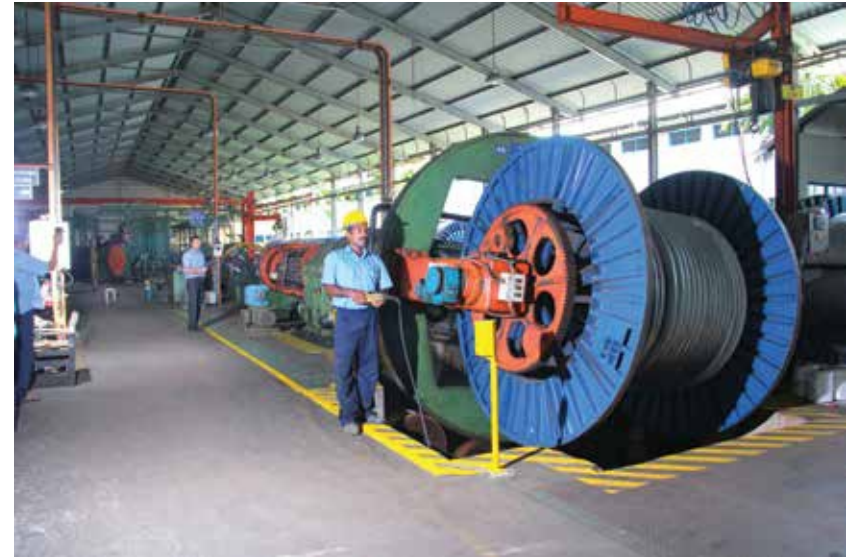
Drum Twister Machine for the assembly and armouring of Power Cables
