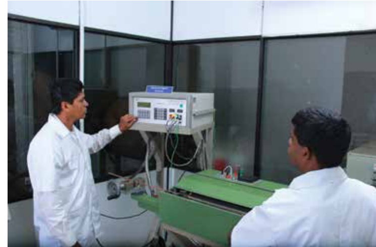
High precision automatic Resisrana Bridge used for the measurement of electrical resistance of Power - X Cables up to 1000 \text{ mm}^2
