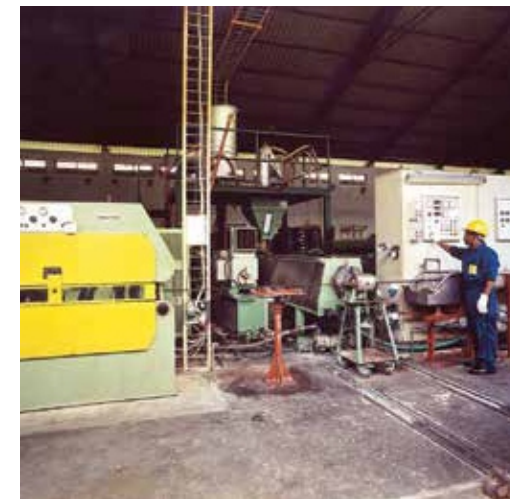
Extrusion of outer sheath of 4x400mm 2 at the rate of 800kg of PVC per hour on an 120mm Extruder.
