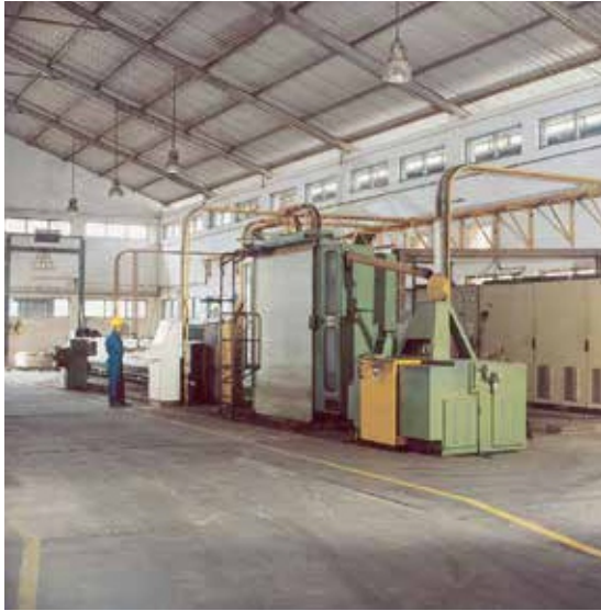
Annealed Copper without dust being drawn at 30m/sec on 15 draft angular shaft. Separate motor driven Sictra rod break down machine
