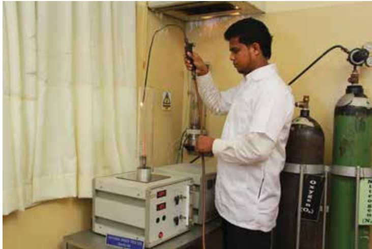
Oxygen index and temperature index tester for the testing of fire retardant properties of low smoke halogen free power cables.
