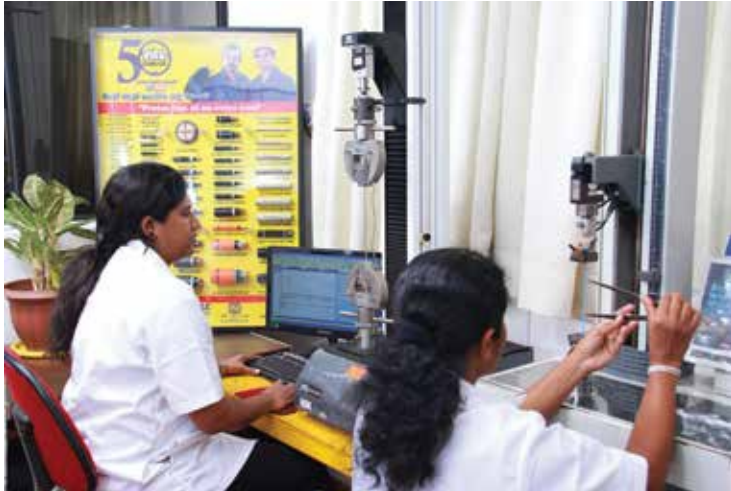
Electronic Tensile Tester - To Obtain tensile strength & elongation values of Power - X Cables up to 4 \times 400 \text{ mm}^2 .
