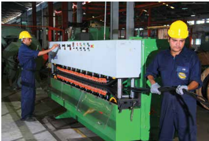
Heavy duty, high boddin weight, Planetary Strander line for assemblies of LA / MV Aerial Bundled Cables
