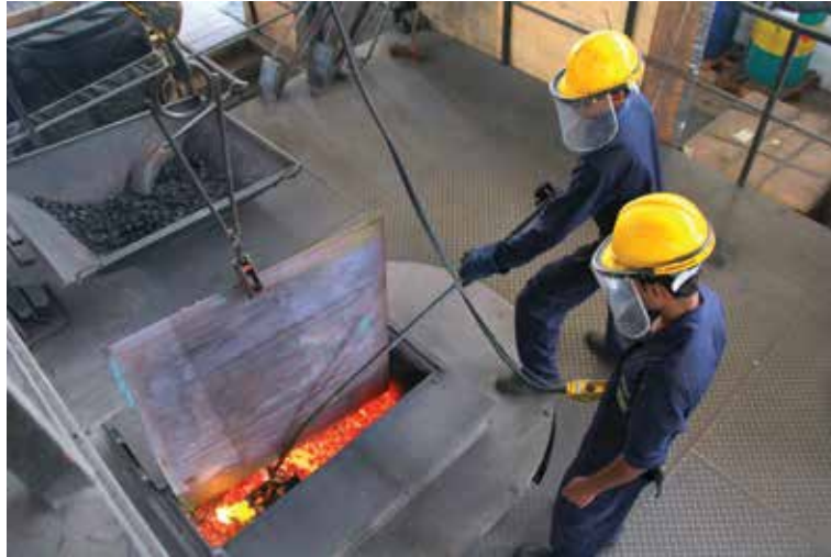
12 channel copper upward casting induction furnace for the manufacture of 8mm diameter oxygen free copper rods .
