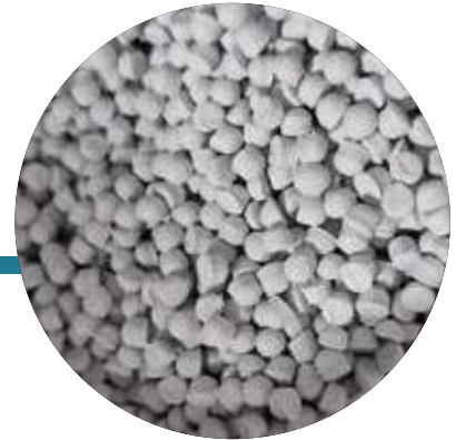
PVC Compound for fire guard cables
